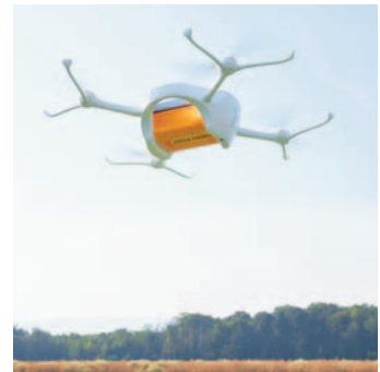
With a load of one kilo and a fully-charged battery, a drone today can manage around ten kilometres.
